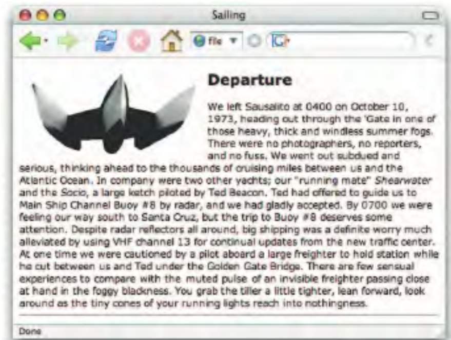
Figure 13-2 You can flow text around an image by using the ALIGN attribute of the <IMG> tag.
