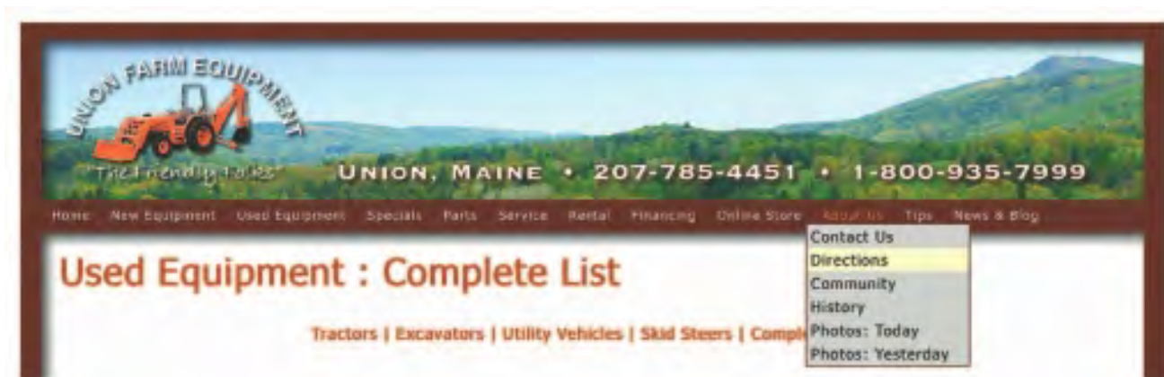
Figure 10-6 Drop-down menus at web sites are built using a combination of HTML, CSS, and JavaScript.
