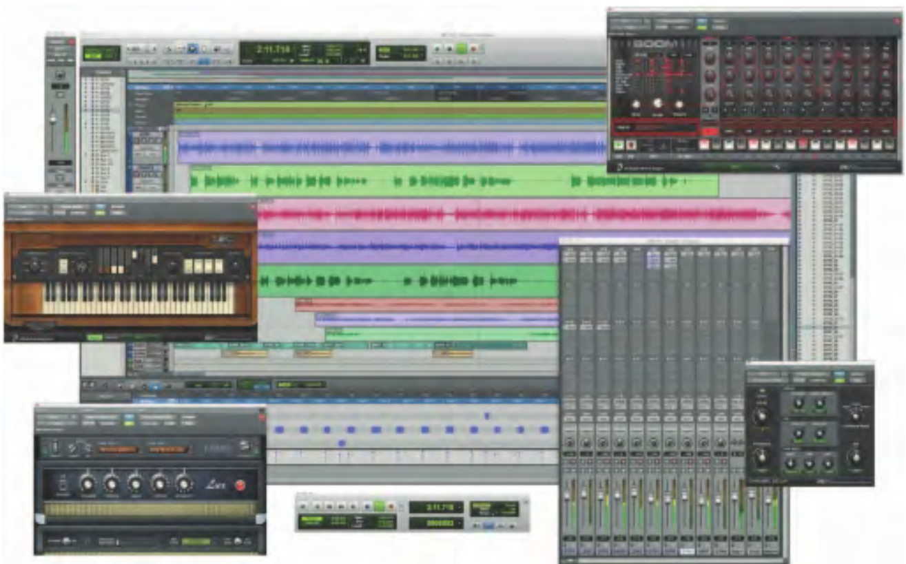
Figure 4-6 Sequencer software such as Pro Tools allows you to record, edit, and save music generated from a MIDI keyboard or instruments and blend it with digital audio.
