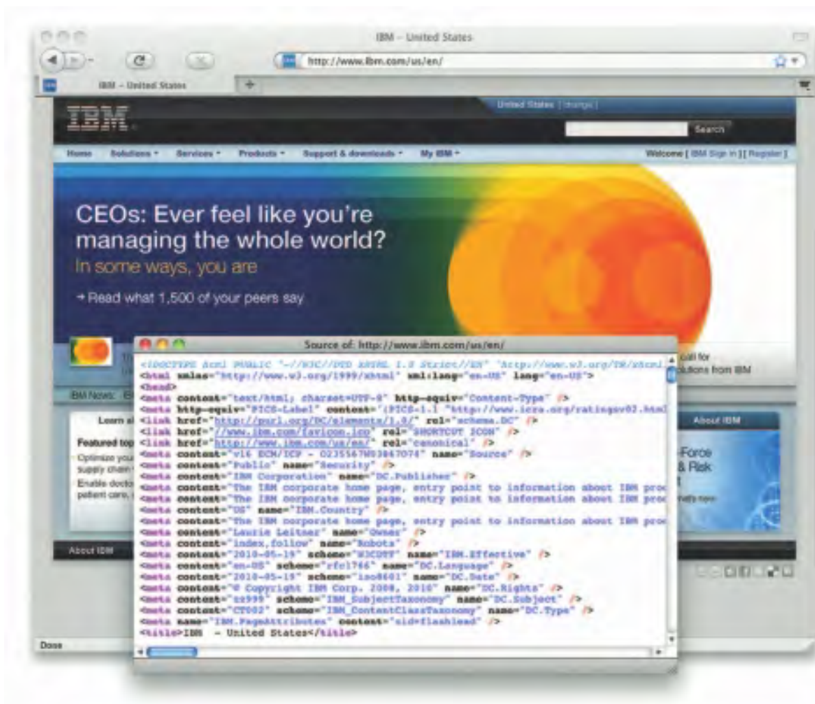
Figure 10-17 Typical copyright and ownership statements embedded in <meta> tags at the top of an HTML page
