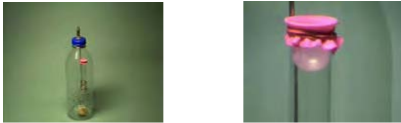
Figures 1 and 2. Plastic bottle with a test tube covered by a rubber membrane
