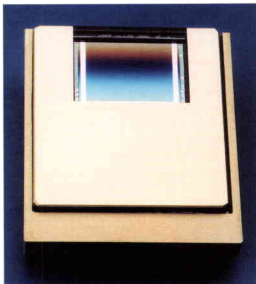
Figure 5. The MERIS CCD
