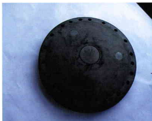
Figure 7. The nose shield before and after re-entry. Note the locations of the three STONE samples
