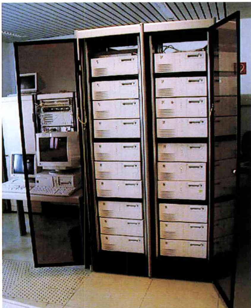
Figure 1. The Linux farm for GOME data processing at the German Processing and Archiving Facility (D-PAF)
