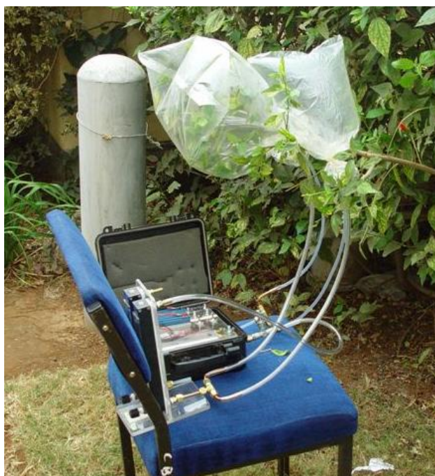
Figure 6.2 A battery powered pump used for trapping volatiles in the field
