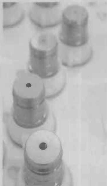
Some of the tungsten apertures used to focus radiation during cancer treatments at Illinois CyberKnife in Park Ridge. | JOEL LERNER -Sun-Times Media
