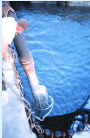
2 The hose of the pump is lowered inside the seine net
