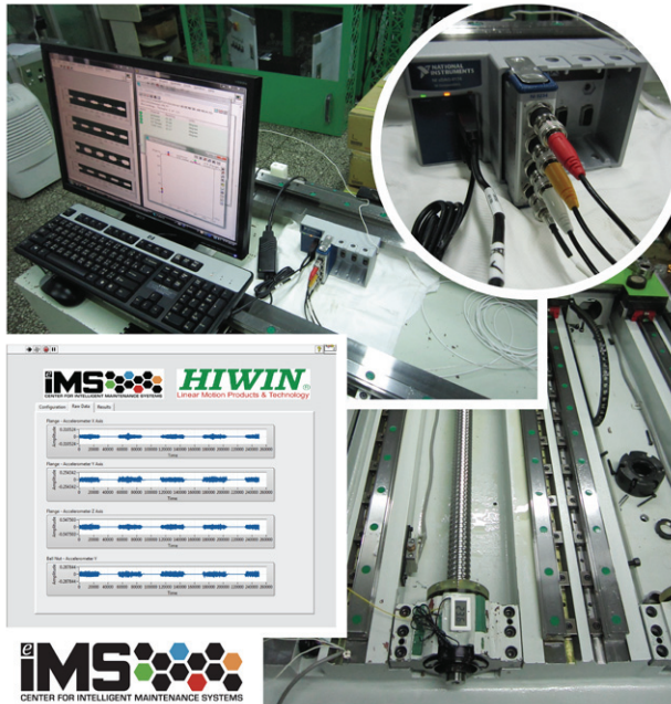
Application of Watchdog Agent® in monitoring ballscrews for precision machining.
