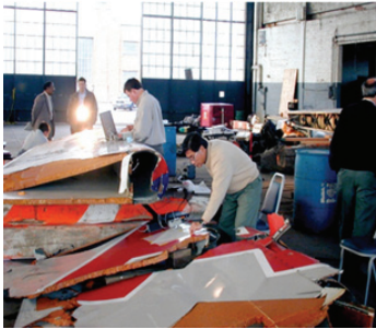
The Computer Aided Tap Tester (CATT) developed by CNDE of Iowa State University was used in the accident investigation of the Airbus A300 (American Airline flight 587) crash in Queens, New York in November 2001. The figures above show the mapping of the damaged rudder and the assembled image.
