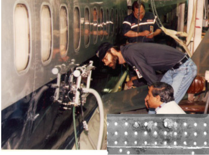
The Dripless Bubbler makes on-aircraft high-resolution images of flaws, damage, and corrosion with a focused ultrasonic beam. The figure here shows the Dripless Bubbler scanning Boeing 747 lap splices.
