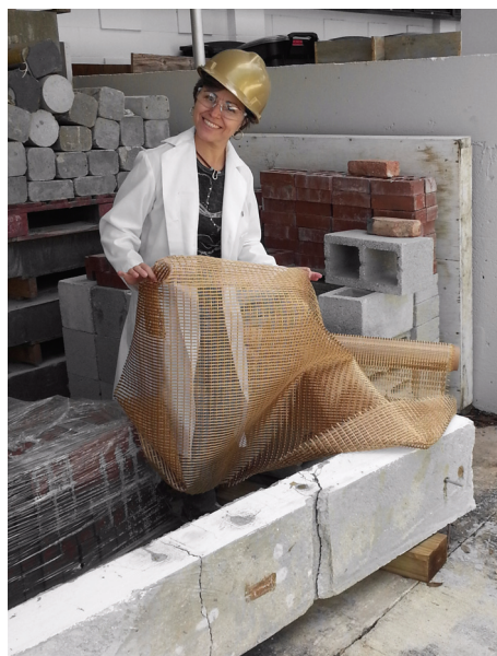
Fabric reinforcement for a concrete surface.
