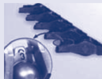
Image 2: Rolling contact rocker arm marking
