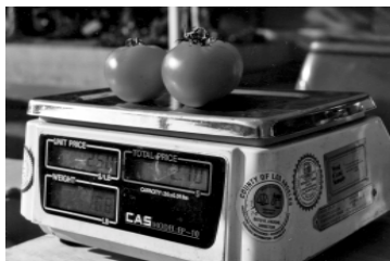
Scale showing various county seals. Scales are verified for accuracy by the Device Division of the Weights and Measures Bureau of each county where the scale will be used.
