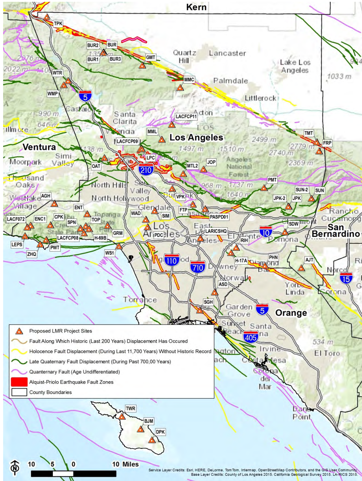
Figure 3.5-1: Mapped Faults within Proposed Project Area
