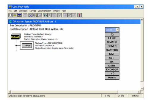
Now add any other nodes to the network that are required and close the window. Finally export the file in the required format, usually binary, for use by the PLC or other PROFIBUS DP Master. The master now searches for the RHE15 RHEONIK on the PROFIBUS DP network and when found connects to it and starts transferring the variable blocks. The red LED on the device slowly stops blinking and goes off when the data exchange is O.K. and the green LED lights up.
