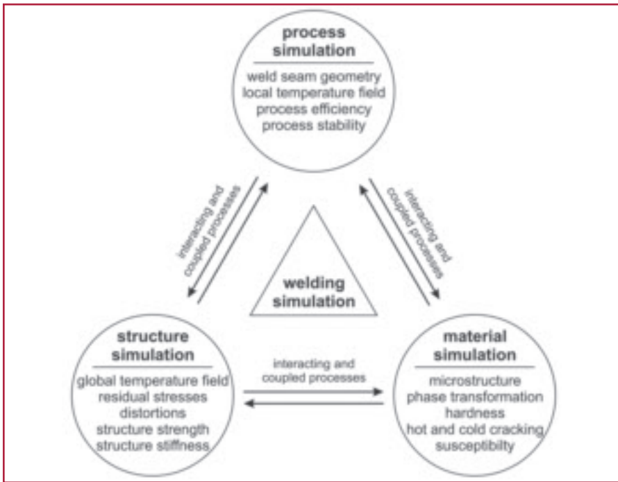
Fig. 1 — Subdomains of welding simulation showing the main target and coupling factors, with reference to Radaj (Ref. 7).
