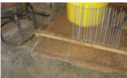
Fig. 2 — In the institute's welding fabrication shop, 6013 electrodes are coated in molten paraffin wax to protect the flux from water before the diver/welder strikes an arc.
