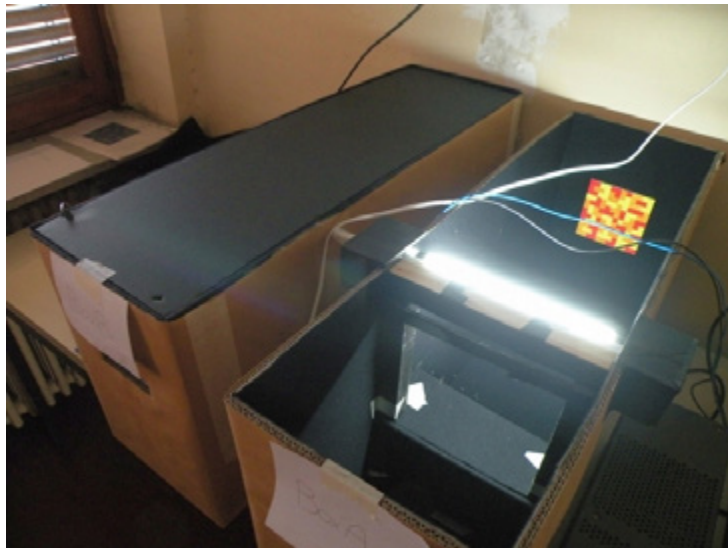
Figure 2 - the two observation boxes with the warm paints on. Note the fluorescent tube that lights the paint
