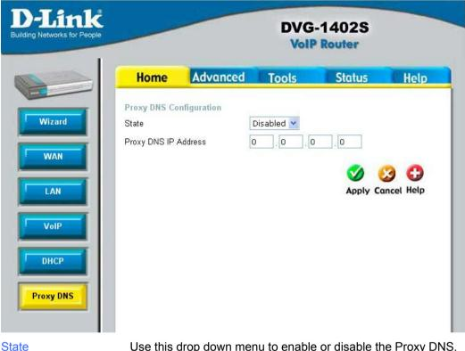
Use this drop down menu to enable or disable the Proxy DNS. Proxy DNS IP Address Enter the IP Address of the Proxy DNS.
