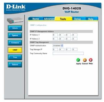
Use SNMP to configure system features for proper operation, performance monitoring, and detection of potential problems in the Router or network.
