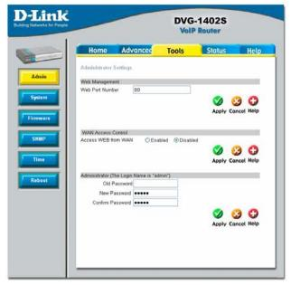
Web Port Number The port number used to access the Broadband Router. The default port number for web management is 80.
