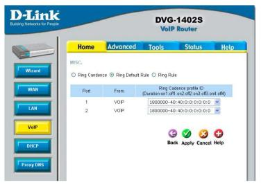
Ring Cadence Profile ID Use this pull-down menu to select a Ring Cadence for the Ring Default Rule. The 8 different Ring Cadences can be configured on the Ring Cadence window.
