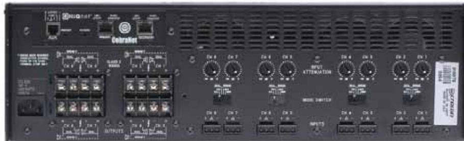
CTs 8200USP/CN Back Panel (note USP/CN CobraNet module at top left)
