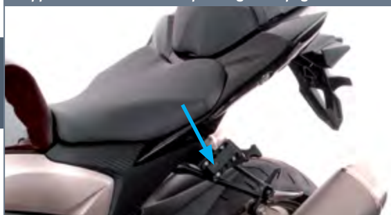
Support arms snap into holders in seconds
