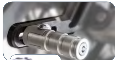
Toe lever is approx. 2.25" (57mm) long without extension
