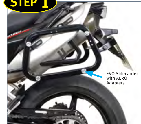
Install an SW-MOTECH EVO, Givi, or Hepco-Becker sidecarrier with Aero adapters on your bike
