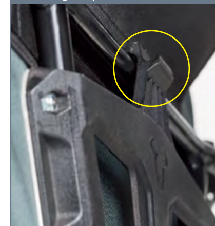
Saddlebags snap onto sidecarriers
