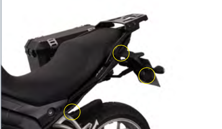
Thumb-sized mounting points remain on the bike when carrier is removed
