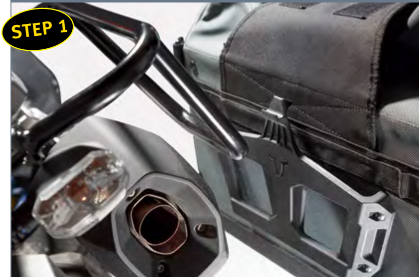
Slide saddlebags on from bottom
