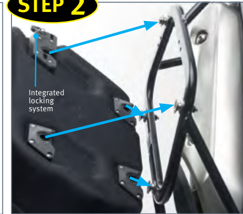
Slide the AERO sidecase onto the mounting points on the sidecarrier, clicking it into place.
