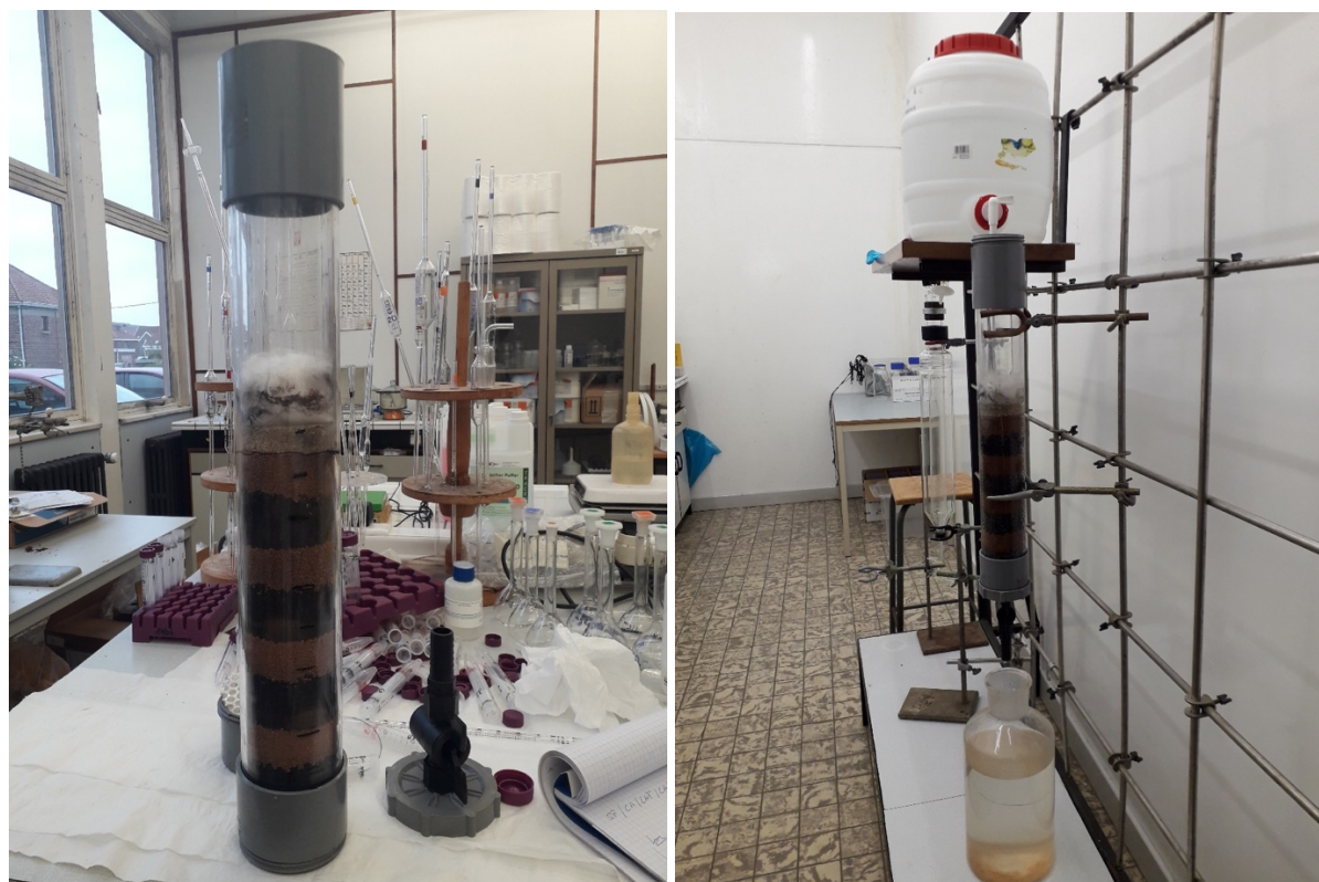
Laboratory scale studies of the removal of arsenic in water solutions percolated through columns of adsorbent materials (repeating layers of laterites and activated carbon). (Courtesy of IPICS BUF:02)
