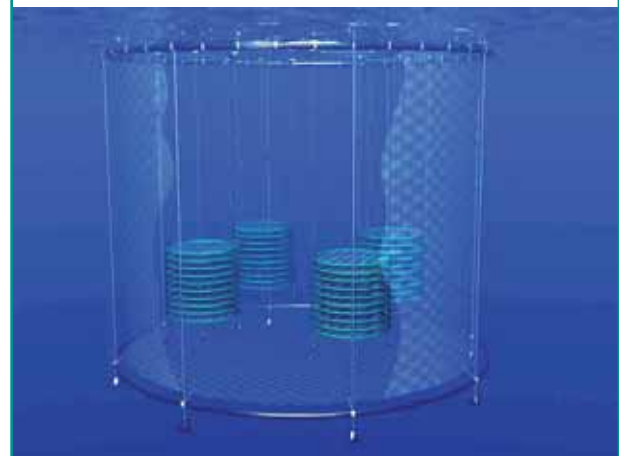
FIGURE 13 Example of cage adapted for flatfish
