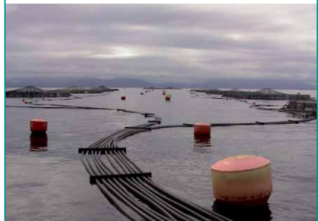
FIGURE 12 Feed is conveyed to individual cages from the silo via compressed air
