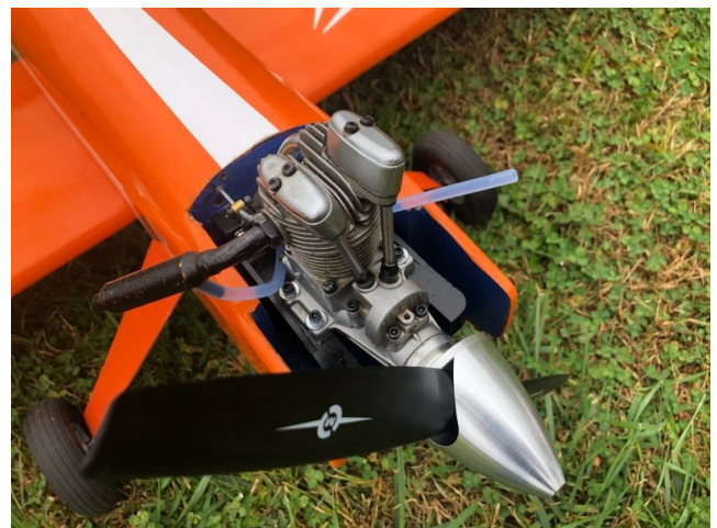
Saito 72 with black exhaust pipe. Tru-Turn Ultimate aluminum spinner. Note the detail of the painted firewall.
