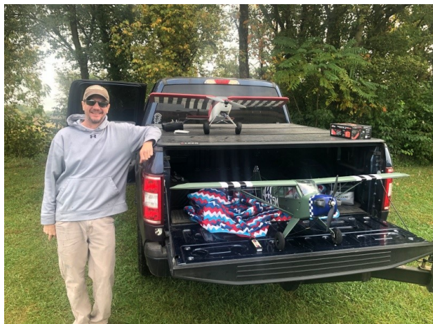
Marshall White proudly shows off two of his planes including his modified Eflite Timber, made to look like a Decathlon, and his other plane is L-4 Grasshopper made by Nexa as an ARF balsa model. The Nexa L-4 incorporates a Rimfire 42 electric motor and 4S battery.
