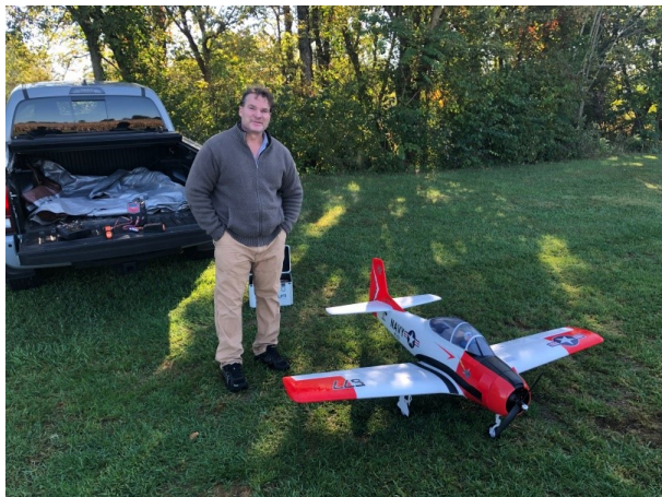
Tim West and his E-flite T-28 2.0m Giant-Scale Foam Monster with a 100amp ECS, 6S 50c LIPO, and Power 60 motor, this sweet bird looks good in the air and is very scale with working flaps!
