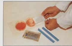
Place petri dishes with single sachet into a Pouch-Bag. (Use 2 sachets for PouchKeep.)
