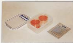
Place either standard petri dishes or MIC test panels in a Rectangular Jar. Prepare multiple sachets for a larger jar.
