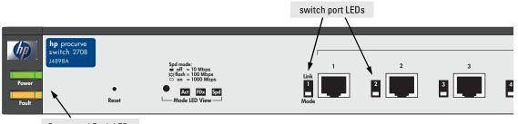
Power and Fault LEDs
