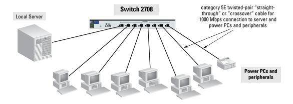
The Series 2700 Switches are designed to be used primarily as desktop switches to which end nodes for power users, local servers, and printers and other peripherals are directly connected, as shown in the above illustration. Notice that the end node devices are connected to the switch by "straightthrough" or "crossover" twisted-pair cables. Either cable type can be used because of the IEEE Auto MDI/MDI-X feature on the Series 2700 Switches.
