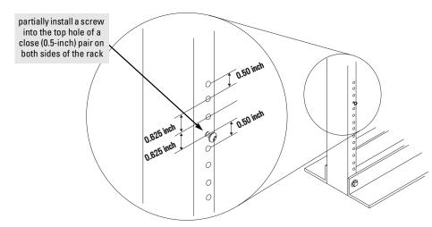
3. Place the switch in the rack and lower it so the notches in the bottom of the bracket slide onto the screws, then tighten these screws.
