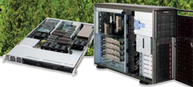
GPU-Enabled Systems 2 GPUs in 1U & 4 GPUs in 4U
