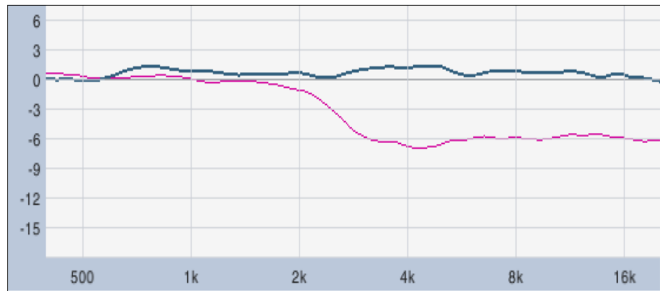
Fig 6.1-2 On-axis vs vertical 35° off-axis response
