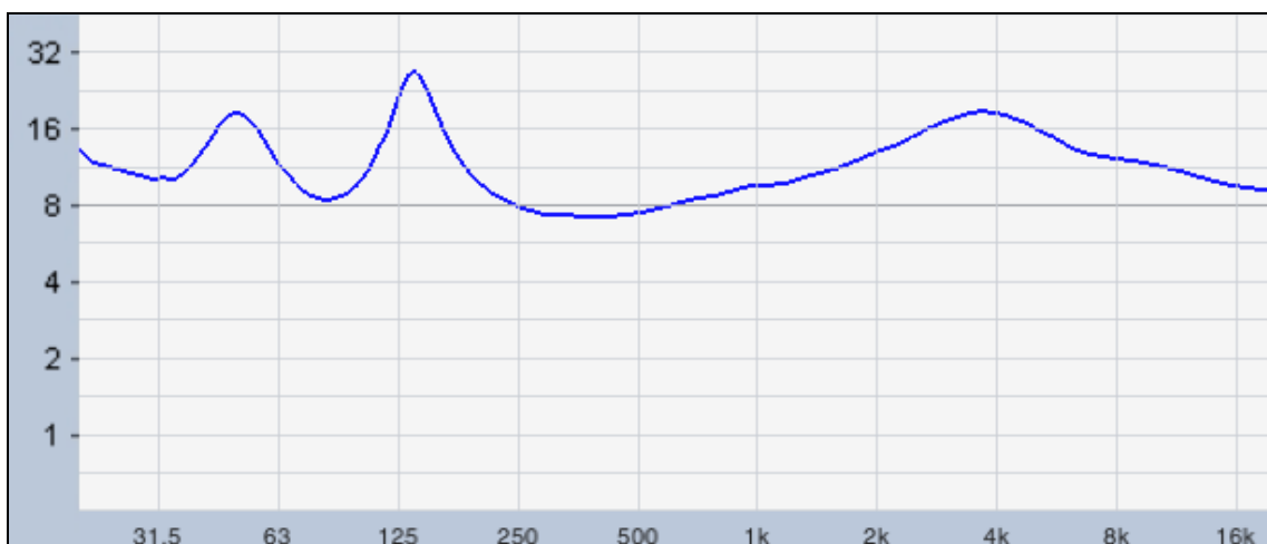
Fig 8.2-1 F101 half-space, 1/12 th octave impedance (ohms) vs frequency (Hz)
