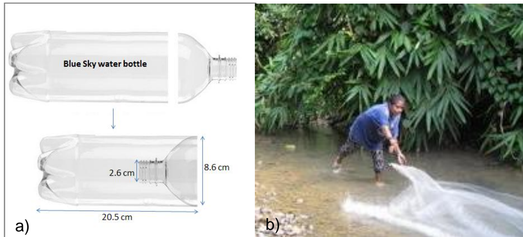
Figure 3.1. Fish trapping methods. a) Blue sky water bottles had the top removed and inverted to create a trap. Five holes were made in the bottom of the bottle to allow for some water flow and traps were tied to vegetation on the stream bank. b) Photo of Research Assistant, Maria, throwing a cast net at OP2 stream.
