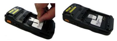
4. First insert the bottom (contacts) and then the upper side of the battery pack into the slot. Press until the battery latch clicks.
