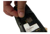
4. Shift the card to the right to lock it into the cardholder; close the card slot:
