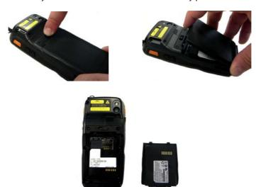
3. Install the new battery pack, first insert the bottom (contacts) and then the upper side of the battery pack into the slot. Press until the battery latch clicks.
