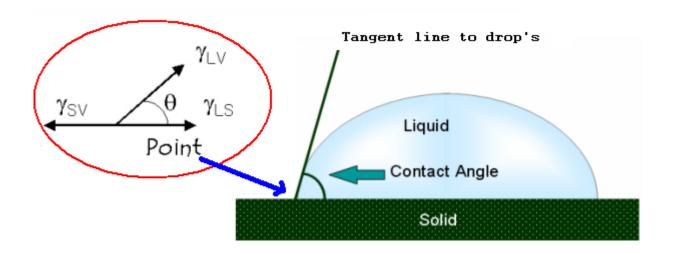
Figure 1. Schematic of a sessile-drop contact angle system
