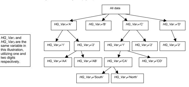
Figure 4.3. Homogeneity groups in an hierarchical tree-structure
