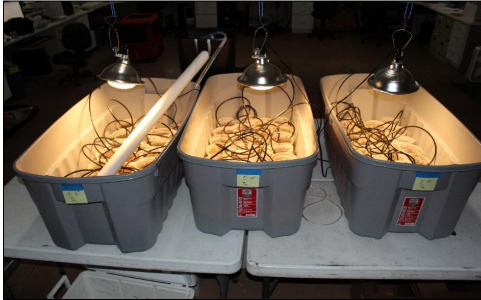
Fig. 10: Laboratory microcosm experiment: the three large chambers contain water baths maintained at each of (right to left) 5°C, 12°C, and 20°C. A total of 32 1-L microcosm chambers were placed together in a large containers, and each microcosm contained 1:1 volumes of clean Colorado River sand and water. Sixteen containers in each temperature treatment contained Chara , half (eight) of which were aerated using aquarium pumps and hosing.
