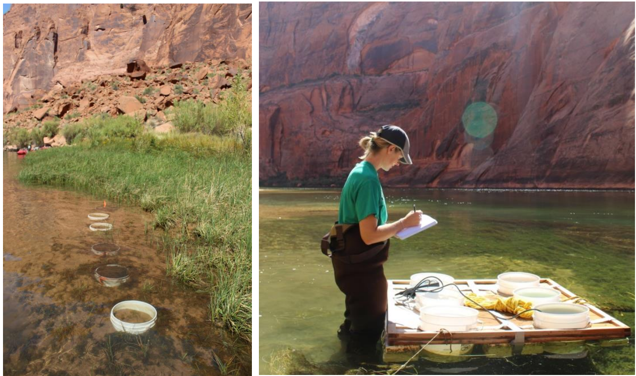
Fig. 9: BHA development field experiments. Floating chambers (right) were used to eliminate fluctuating flow impacts on BHA development, against controls in shoreline chambers (left) that were subject to daily flow fluctuations, and boat wake and wind wave impacts. Three of the six chambers in each treatment contained Chara , while the remaining three contained only non-BHA shoreline sand and mainstream water. Water quality measurements and presence of BHA were measured initially and at 38 days during the course of the experiment.
