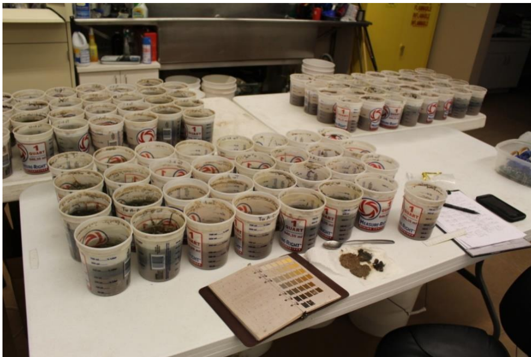
Fig. 11: Laboratory microcosm experimental 1 L chambers at the conclusion of the 10-day experiment (Fig. 10). Depth of BHA development and sediment color was measured in each of the treatment combinations.
