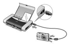
The icon will display on the LCD display of the digital camera when the printer is correctly connected.
