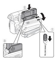
1 Slide OPEN/EJECT fully in the direction of the arrow and open the cassette compartment cover.
