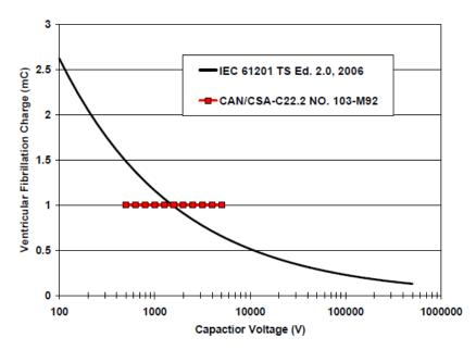
Figure 6. Capacitor Charge that causes Ventricular Fibrillation (IEC 61201) compared to 1 mC standard for Electric Fences in CAN/CSA C22.2
