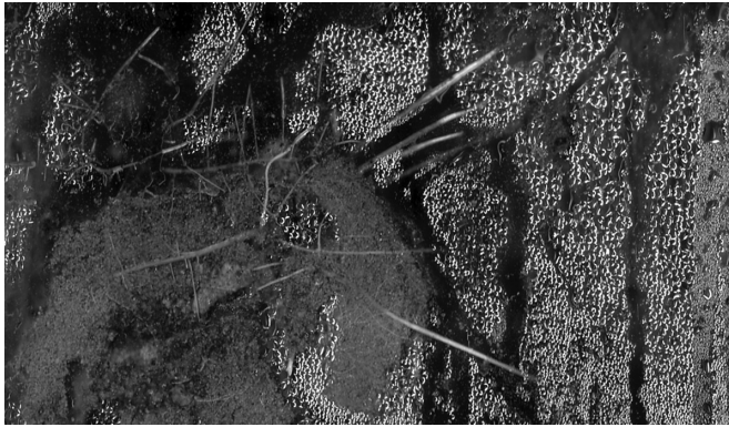
FIGURE 42.2 Picture section within an inappropriately installed MR-OT (90°) 3 months after installation (soil corer). The picture was captured with a scanner MR (CID, Cedar Rapids, IA). The roots of Fagus sylvatica can be seen to grow toward soil voids; many regions of the picture are obscured by condensed water in alternation to voids.
