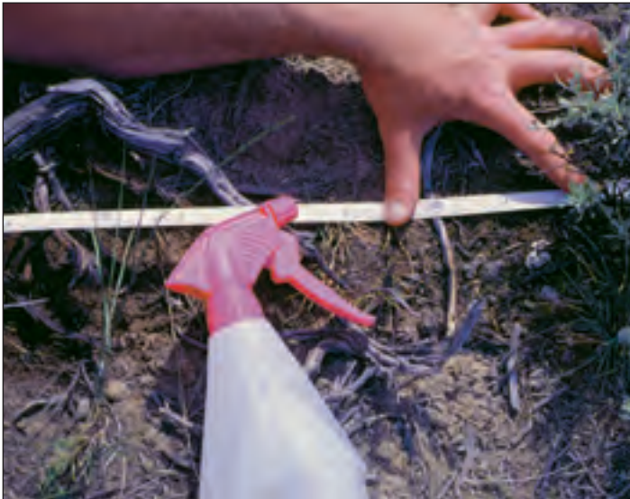
Figure 6.3 Use of line-intercept for measuring biological crust cover along with other community attributes (vascular plant cover, litter, bare mineral soil, rock). Note the placement of the transect line close to the soil surface. Cover of each entity is measured along the top edge of the tape. A misting of water makes crustal organisms more visible and therefore easier to measure.
