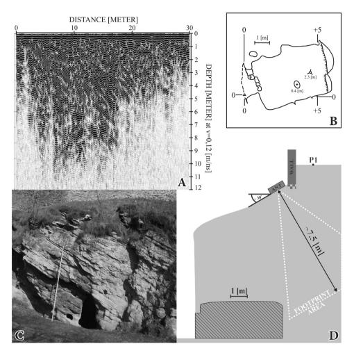
**Figure 4.** *A* – Radargram fragment from the profile number 15 imaging stratification and cave's ceiling. *B* – Plan of the Szydło's Cave I (Gubała et al., 1998). *C* – Opening entrance of the Szydło's Cave I with a visible stratification of limestone (a 4 m geodesic patch makes it easier to assess the size scale). *D* – Scheme showing the methodology of measuring on escarpment and the way electromagnetic waves spread.
