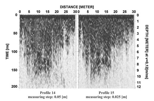
Figure 2. Radargrams fragments from profiles 14 and 15 documenting differences between GPR recoding, depending on the type of the measuring step.
