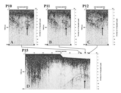
**Figure 3.** Selected radargrams received as a result of imaging with the use of shielded antenna 250 MHz showing the anomalous areas and forecasting occurrences of voids or loosening in rock mass transformed by the karst processes.
