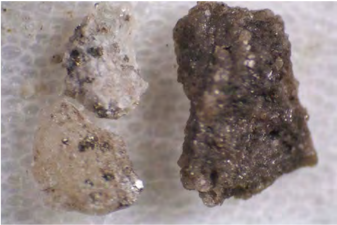
Binocular microscope image (2500x) – Pure Lisbon 814-A (Map #31), 8910-15 feet, dolomite cuttings, the large sample containing intercrystalline porosity, the two small samples showing sulfides.
