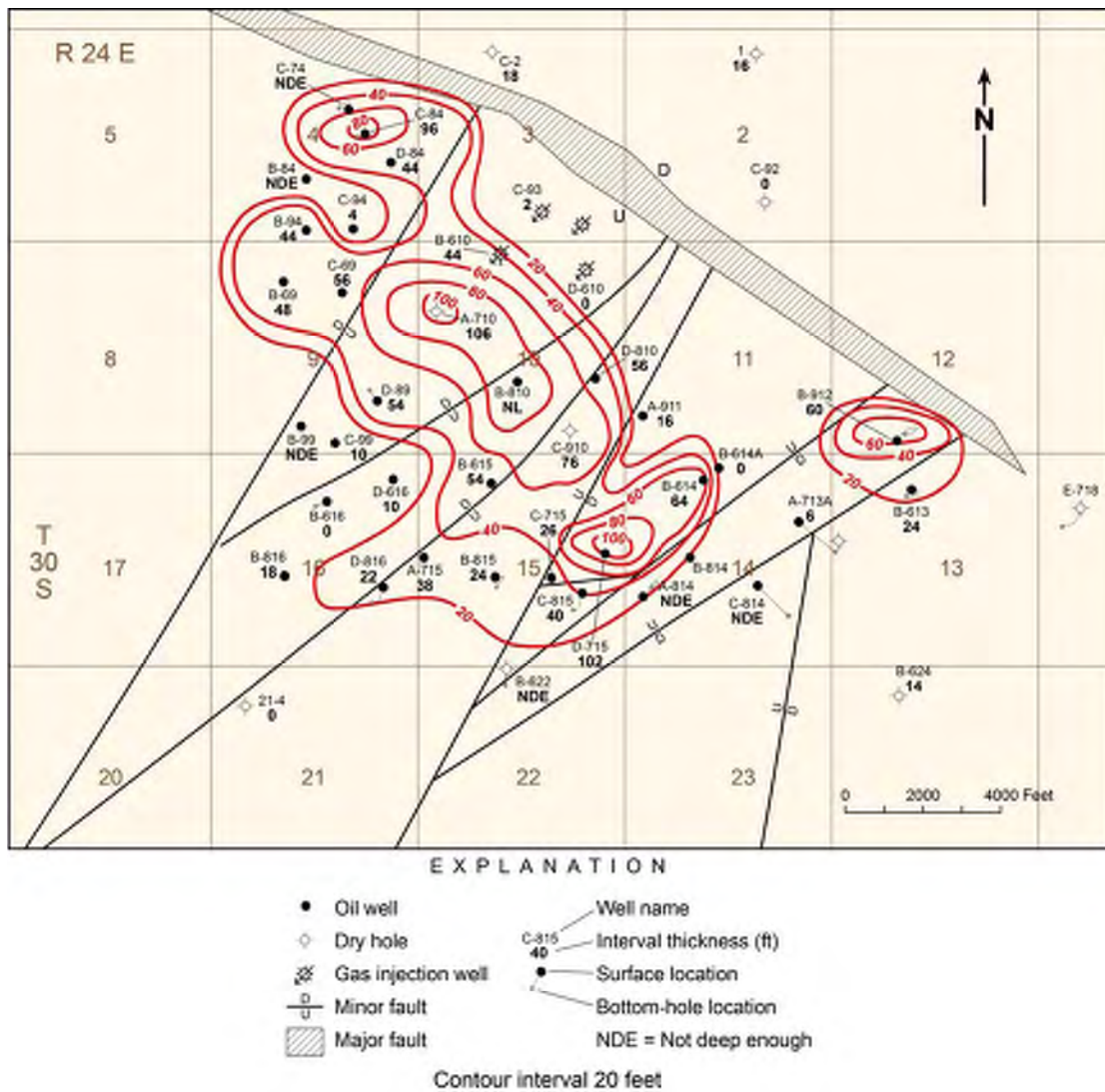
Figure 2-9. Net feet of porosity isochore for reservoir zone 2, Leadville Limestone, Lisbon field.
