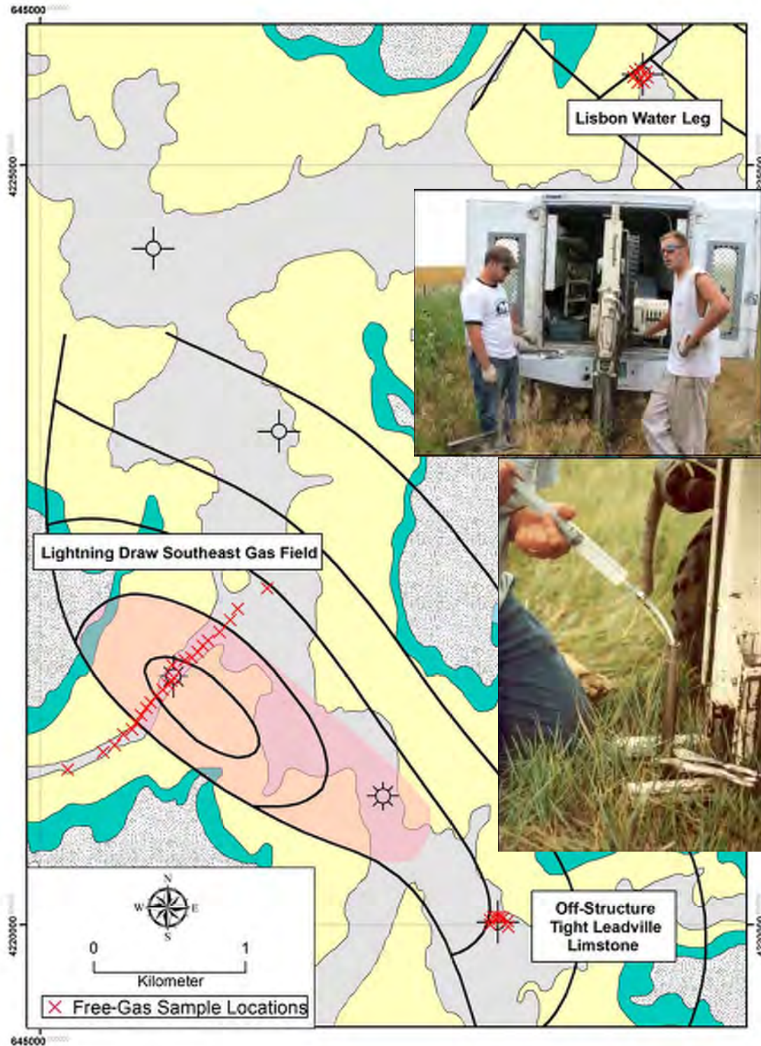
Figure 5-15. Location of 6-foot-deep free-gas samples over and off Lightning Draw Southeast field (shown in pink). The samples were collected with a Geoprobe “Direct-Push” drill and gas was extracted through plastic tubing (inset photos), which was inserted into the 1-inch steel pipes. Surface geology modified from Doelling (2005); see figures 5-1 and 5-11 for explanations of well symbols and geologic units. Form line contours based on structure contour map of the Leadville Limestone shown on figure 5-5.
