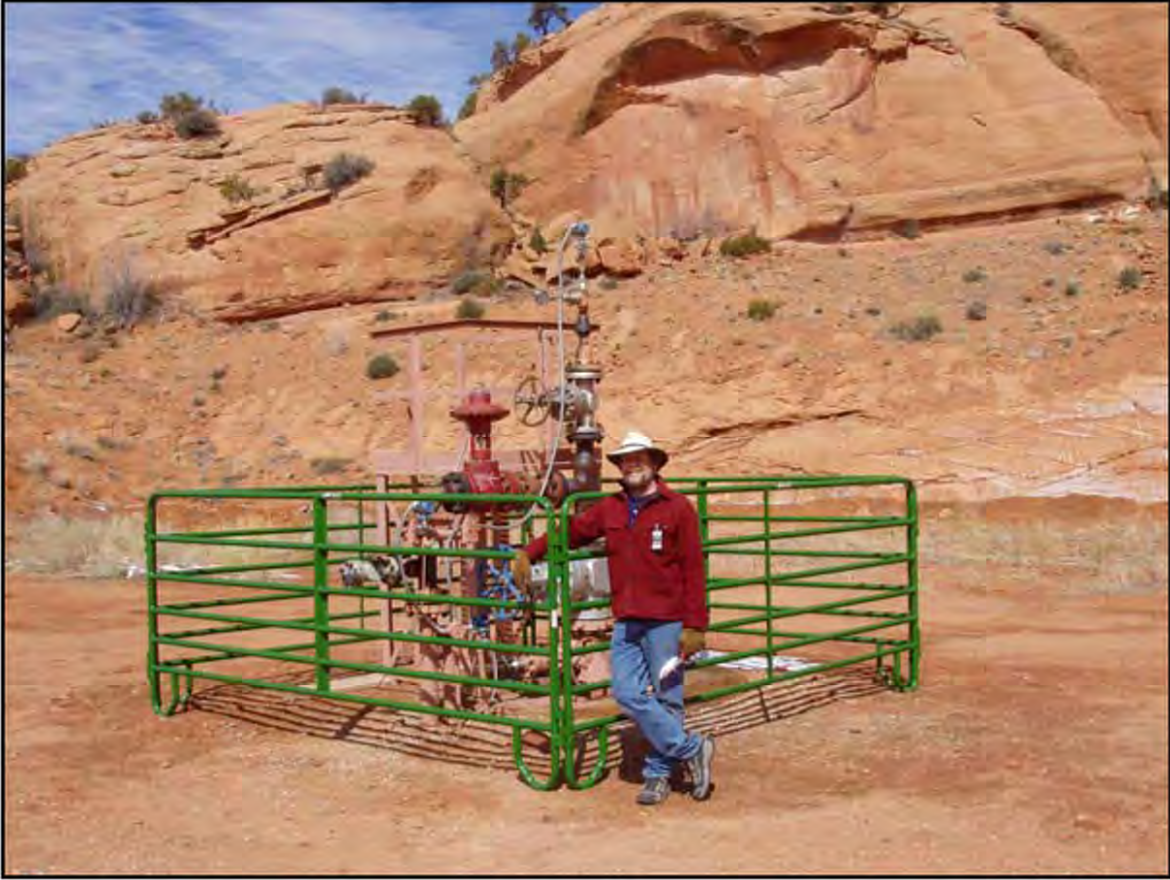
Figure 5-13. The Lisbon No. C-910 well, which produces 7 MMCF/D of low-Btu ( \approx 670 ) sour gas with considerable amounts of N_2 and CO_2 (see table 5-1). Soils samples were collected from the ledge above the well pad to avoid contamination.
