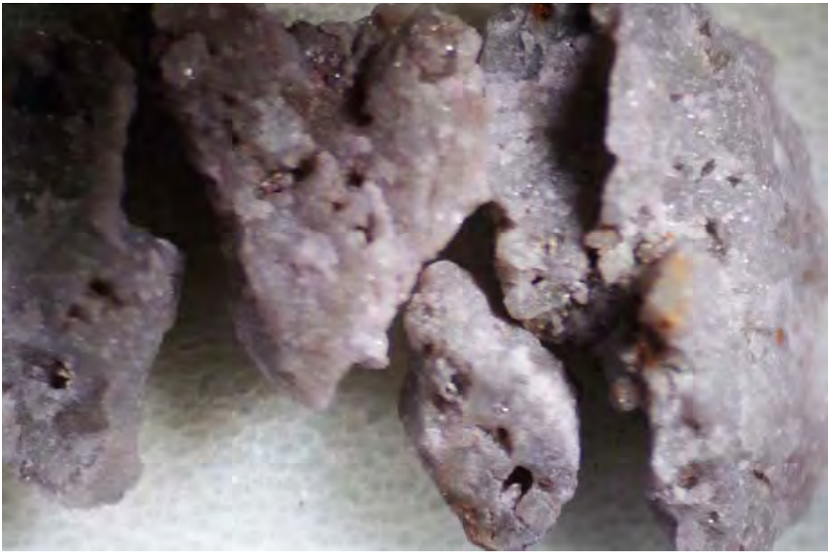
Binocular microscope image (1400x) – Richfield Hatch Mesa 1 (Map #26), 7810-20 feet, representative samples with crinoid moldic porosity and mini-vugs in medium crystalline dolomite.
