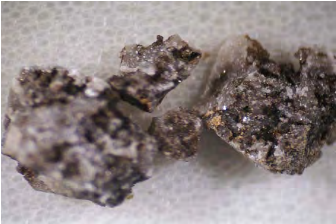
Binocular microscope image (1500x) – Pure Big Flat 3 (Map #19), 7721-22 feet, representative samples showing oil-stained porosity and bitumen (bladed) in medium crystalline dolomite.
