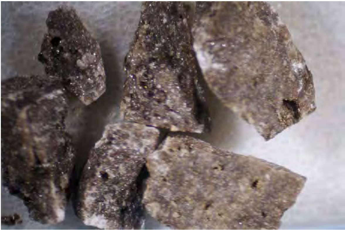
Binocular microscope image (1200x) – Pure Big Flat 3 (Map #19), 7719-20 feet, low porosity dolomite samples selected for epifluorescence grading.
