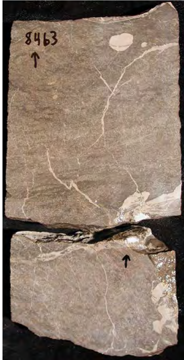
Figure 3-7. Typical peloidal grainstone/packstone representing moderate-energy, "hard" peloid shoal lithofacies. Lisbon No. B-816 (NE1/4SW1/4 section 16, T. 30 S., R. 24 E., SLBL&M [figure 2-1]); slabbed core from 8463 feet.
