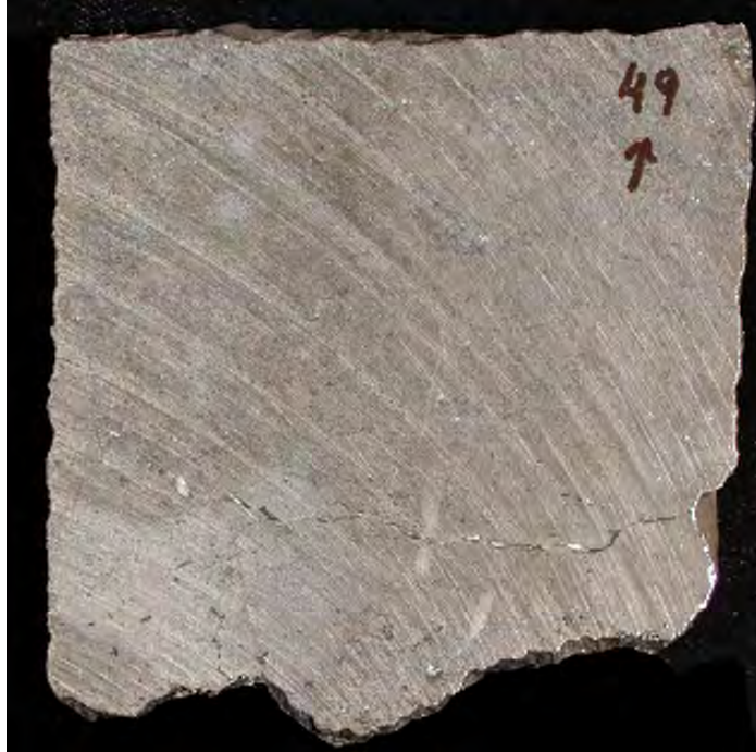
Figure 3-8. Typical skeletal/“soft” peloidal wackestone/mudstone representing low-energy, restricted-marine, middle-shelf lithofacies. Lisbon No. B-816 (NE1/4SW1/4 section 16, T. 30 S., R. 24 E., SLBL&M [figure 2-1]); slabbed core from 8549 feet.
