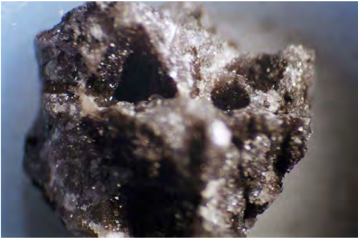
Binocular microscope image (2400x) – Pure Big Flat 3 (Map #19), 7714-15 feet, large cutting with rounded vugs and molds (?), dolomite crystals lining large pores. Note probable oil staining and bitumen.
