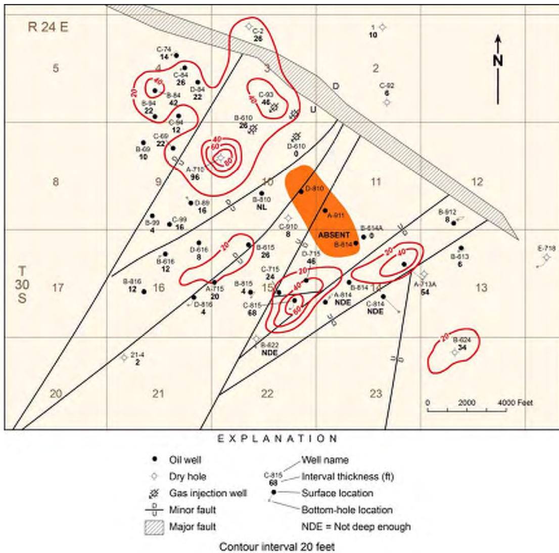
Figure 2-8. Net feet of porosity isochore for reservoir zone 1, Leadville Limestone, Lisbon field.
