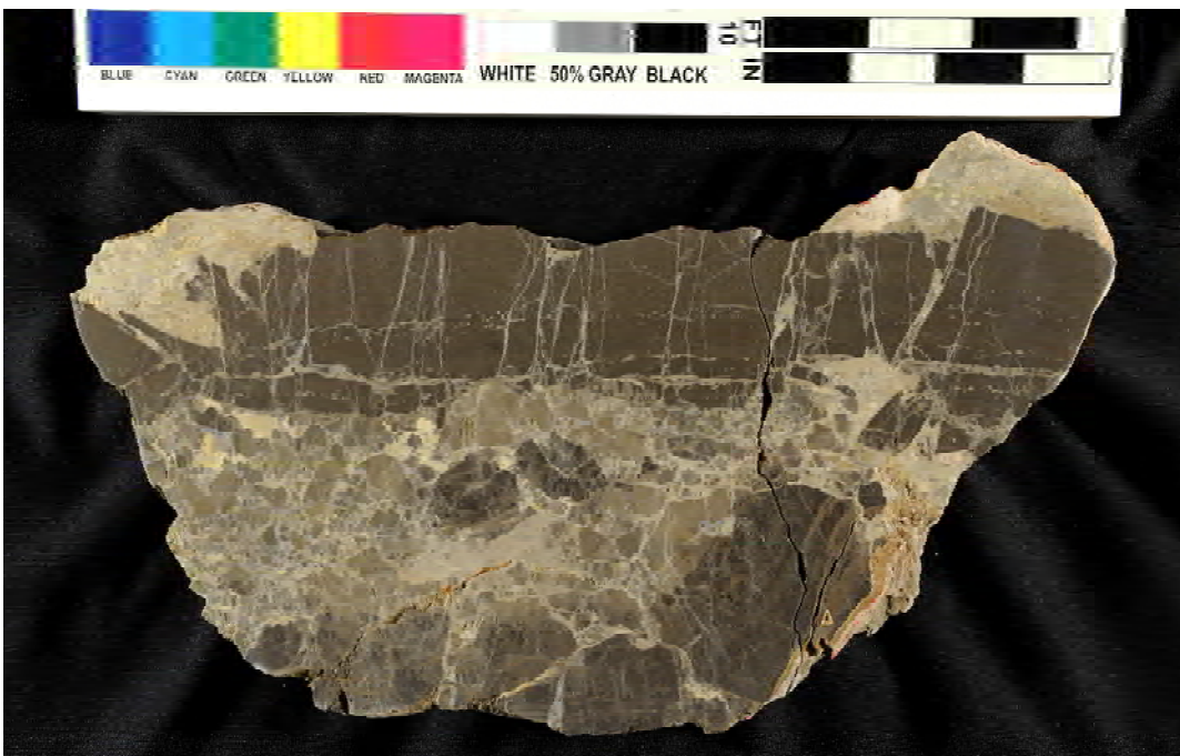
Figure 8-19. Slabbed specimen of highly brecciated rock typical of that present at study site 3.
