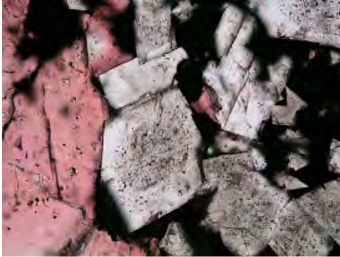
Figure 4-43. Dolomite (colorless) and calcite (red) from the Lisbon NW USA No. B-63 well at 10,004 feet. The cloudy appearance of the dolomite is due to abundant fluid inclusions. Saddle dolomites (center of photo) typically have cloudy cores and clear rims. Width of image is 0.7 mm.
