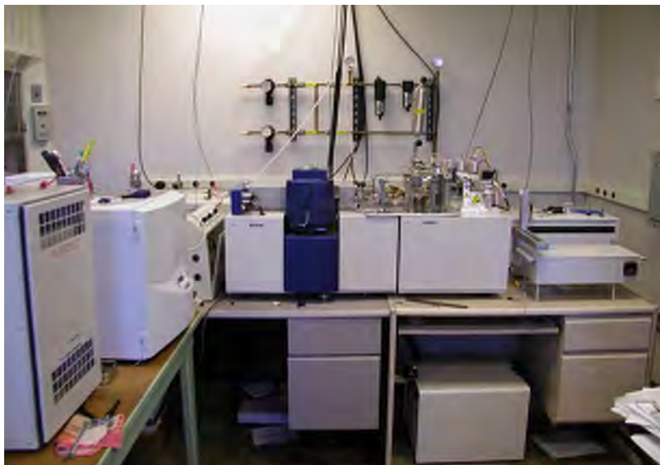
Figure 4-64. The CSM Stable Isotope Laboratory's GV Instruments IsoPrime stable isotope ratio mass spectrometer. Several peripheral devices are interfaced with the IsoPrime for both dual-inlet and continuous flow applications.
