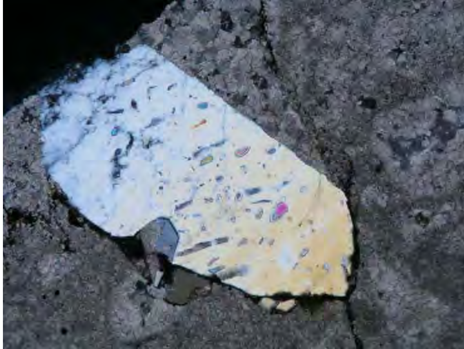
Figure 4-50. Coarse-grained quartz crystal from the Lisbon No. D-616 well at 8356 feet. Small oriented grains of anhydrite are encapsulated in the quartz. Width of image is 1.3 mm.
