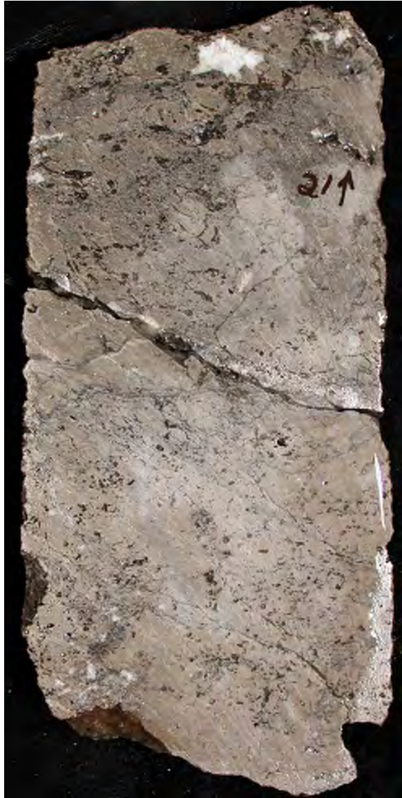
Figure 3-6. Typical peloidal/skeletal packstone/wackestone representing moderate-energy, open-marine, shoal-flank lithofacies. Lisbon No. B-816 (NE1/4SW1/4 section 16, T. 30 S., R. 24 E., SLBL&M [figure 2-1]); slabbed core from 8521 feet.
