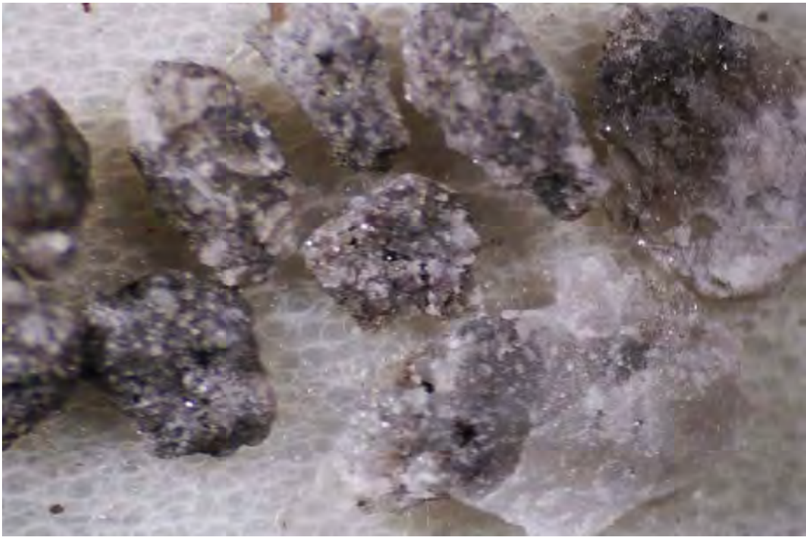
Binocular microscope image (1700x) – Pure Spiller Canyon State 1 (Map #32), 9330-40 feet, samples of dolomite with good intercrystalline porosity and bitumen.
