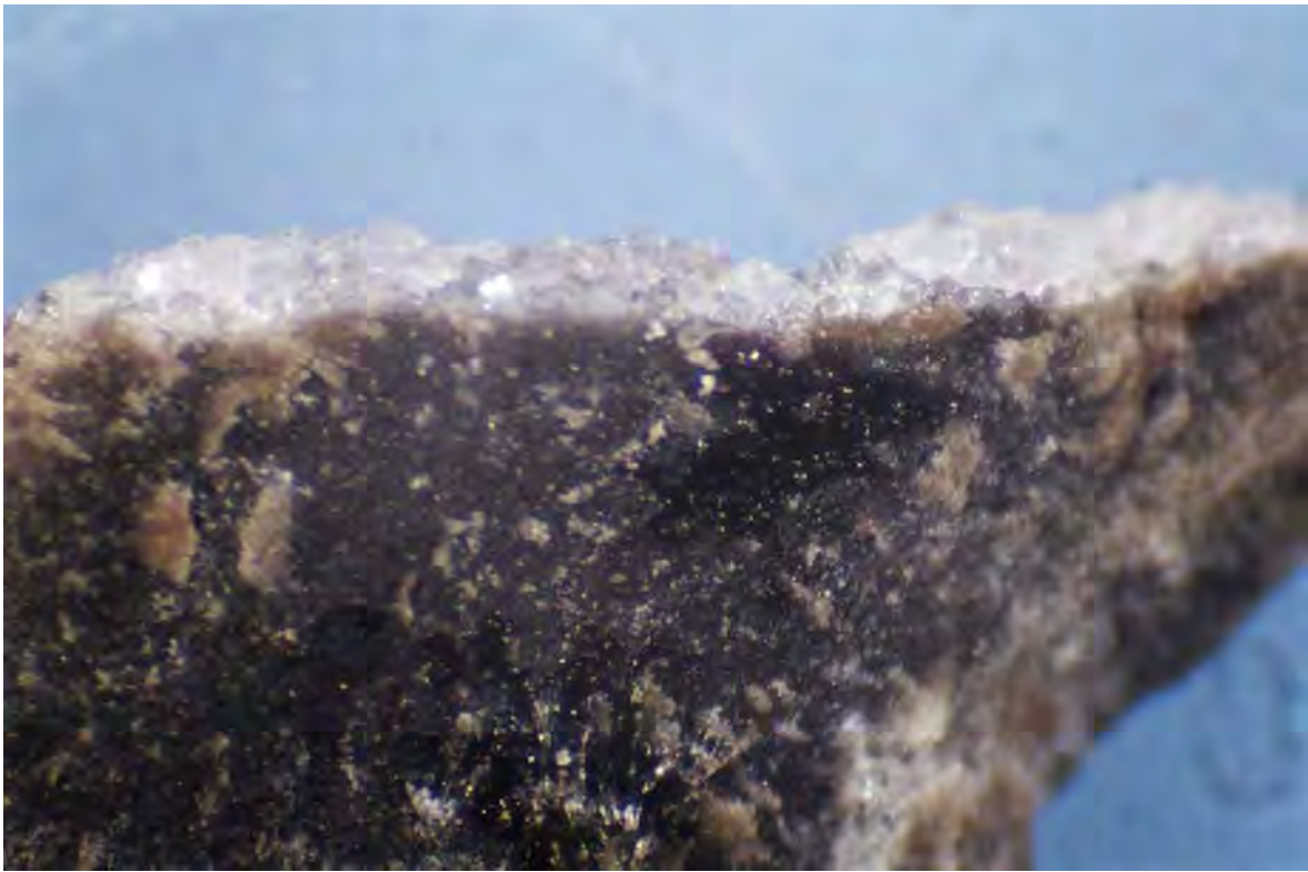
Binocular microscope image (3700x) – Pure Spiller Canyon State 1 (Map #32), 9100-10 feet, dense dolomite cutting with white dolomite crystals lining fracture.
