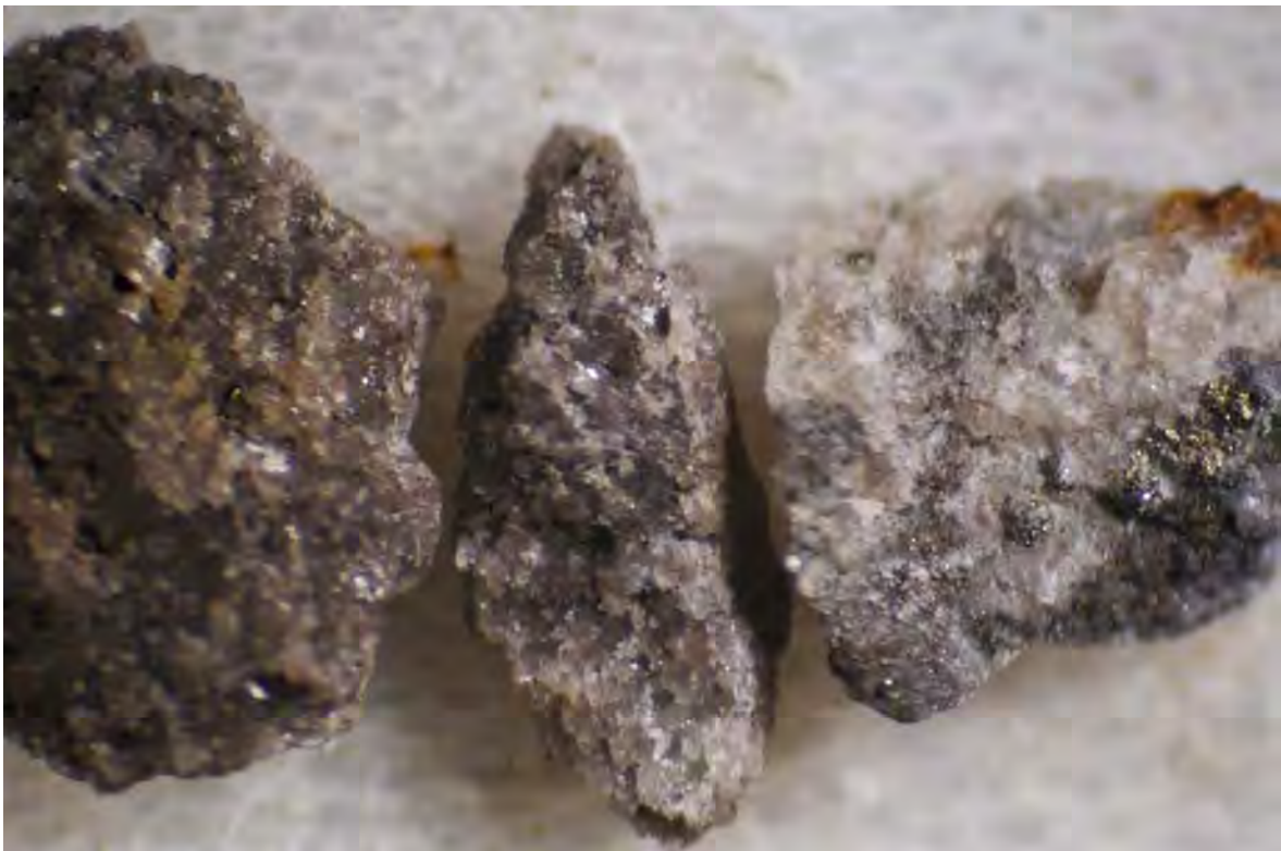
Binocular microscope image (2500x) – Pure Lisbon 814-A (Map #31), 8890-95 feet, three samples with modest porosity, bitumen, and sulfides. Note possible oil stain in the left hand sample.
