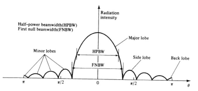
*Half-power beamwidth* (HPBW) is the angle between two vectors, originating at the pattern's origin and passing through these points of the major lobe where the radiation intensity is half its maximum.
