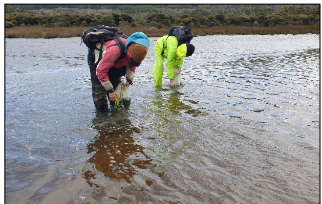
Collection of sediment core (top), measuring aRPD in the core profile (upper middle), transferring the core to a mesh (0.5mm) sieve bag (lower middle) and rinsing the core sieve bags in the subtidal channel (bottom).
