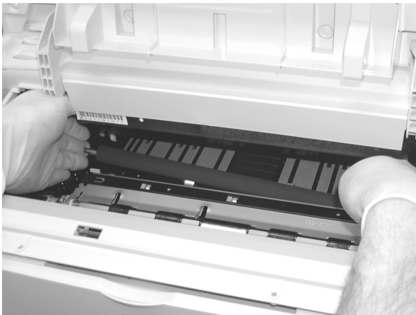
Figure 4 Removing the transfer roller
