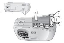
4 Close the battery compartment cover by sliding it into place and then clicking it shut.
