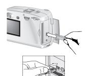
3 Plug the flat end of the cable into any USB port on your computer.
