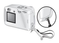
2 Pull the strap through the loop, and then pull the knot tight.
