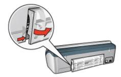
Remove the paper jam from the back of the printer, and then replace the rear access door.
