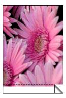
If the border appears above the tear-of tab, then align the print cartridges.
