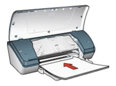
Note: If you are using letterhead, verify that letterhead is facing down and towards the interior of the printer.
