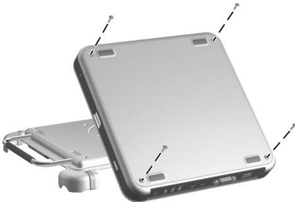
Removing the Top Case Screws
