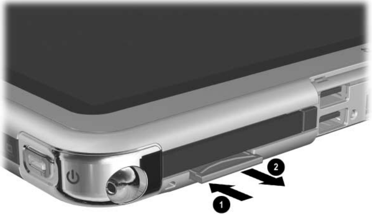
Releasing the SD Card (space saver shown)
