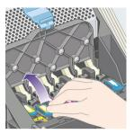
8. Using the blue handle, gently disengage the printhead.
