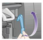
5. Carefully remove any of the jammed paper that you can lift up and out from the top of the printer.
