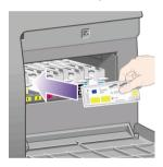
2. When the printhead cleaner has been pushed all the way in, press inwards and downwards as indicated by the arrow shown here, until it clicks into place.
