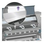
**19.** Carefully pull the rest of the paper down and out of the printer. Look to see if there any loose pieces of paper left in the paper path.
