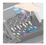
When all the printheads have been inserted correctly and accepted by the printer, the printer will beep.
