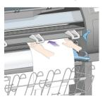
7. Insert the sheet until it reappears from the printer as shown below.
