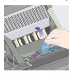
**7.** To remove a printhead, lift up the blue handle.
