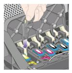
Rub the sponge against the contacts with a light force along the entire depth of the flex connector as allowed by the mechanical stop on the tool.
