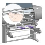
10. Carefully remove the cut-off lower end of the paper.
