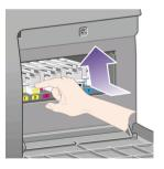
4. Lift up the printhead cleaner to remove it from the slot, and slide it out horizontally as shown below.
