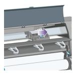
17. Carefully remove any of the jammed paper that you can lift up and out from the top of the printer.
