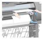
**9.** Align the leading edge of the sheet with the metal bar in the platen.
