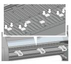
Using the bottle of oil supplied with the Maintenance Kit, insert the pointed end of the bottle into each hole in turn, and put three drops of oil into each hole.
