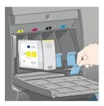
9. Lift the cartridge out of its drawer.
