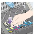
When installing the new printhead there may be some resistance, so you need to press it down firmly but smoothly.
