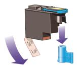
The printhead is designed to prevent you from accidentally inserting it into the wrong position. Check that the colored label on the printhead matches the colored label of the carriage position into which the printhead is to be inserted.
