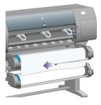
5. Remove the cut-off piece of paper.
