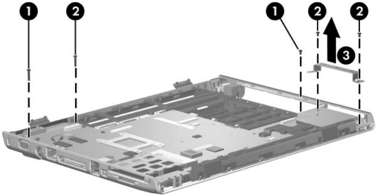
Removing the System Board Screws
