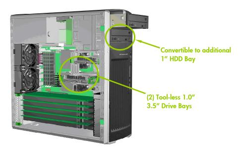
The xw6200 supports (2) tool-less internal 1" HDD slots and (2) 5.25" tool-less optical bays. One of the 5.25" bays can be converted to additional 1" internal HDD bay using the optional DY659A bracket. The xw6200 can support up to 1.5TB of SATA storage (with the Adaptec 1420SA controller), and up to 900 GB of SCSI storage.
