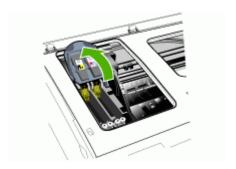
4. Lift the handle of a printhead and use it to pull the printhead out of its slot.
