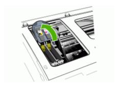
**4.** Lift the handle of the printhead you want to replace and and pull the printhead out of its slot.
