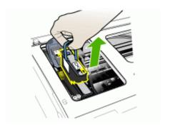
**5.** Before installing a printhead, shake the printhead up and down at least six times while the printhead is still in its packaging.
