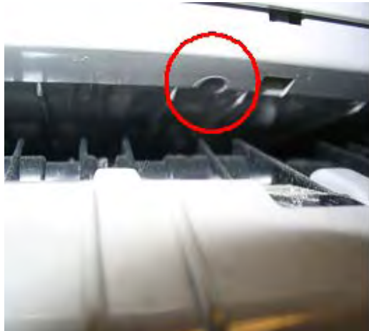
The transmitter optical sensor is located in the upper middle part of the flipper assembly
