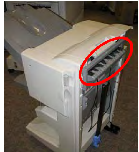
The flipper assembly is located on the side of the multi-function finisher
