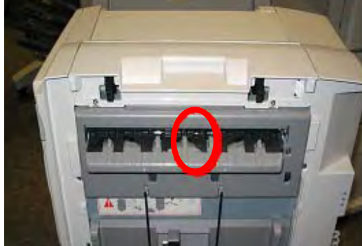
Location of the optical sensors
