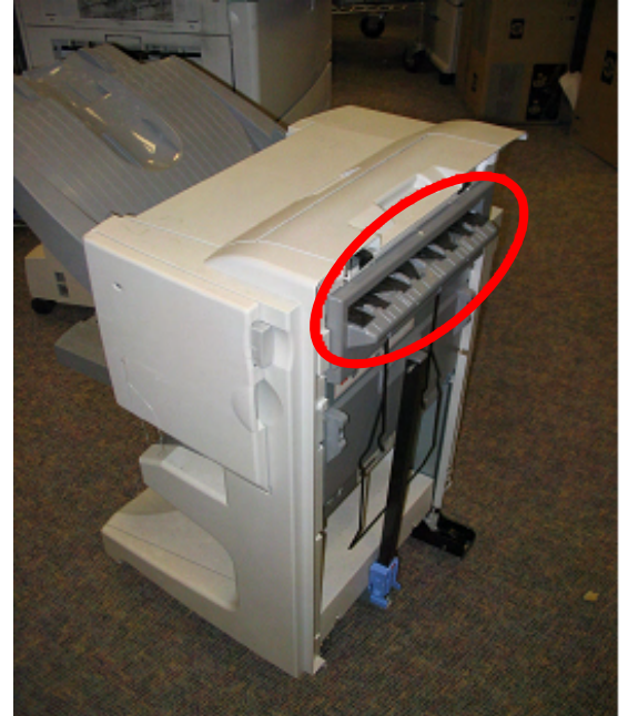
The flipper assembly is located on the side of the multi-function finisher
