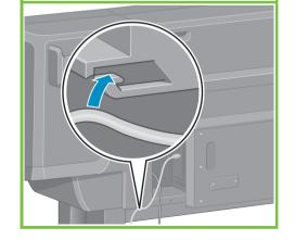
Plug the power cable into the rear of the printer, and then plug the other end into the AC power outlet.
