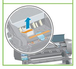
Remove the packing tape that is holding down the printhead carriage latch.
