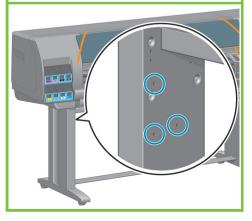
Insert two screws into the two forward holes. Leave sufficient space between the screw heads and the leg to attach the left side of the take-up reel assembly.
