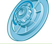
Load the take-up reel spindle into the printer by pushing firmly on each end of the spindle.
