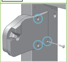
Use four screws to attach the take-up reel deflector supports.
