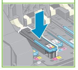
If a "Reseat" message appears on the front panel, check that all of the protective tape has been removed, and then firmly reseat the printheads. If the problem persists, refer to the *HP Start-Up Kit* CD/DVD.
