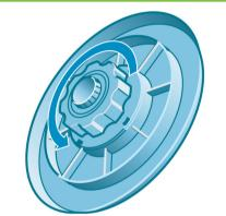
Slide the blue hub onto the spindle. Tighten the plastic nut on the blue hub.
