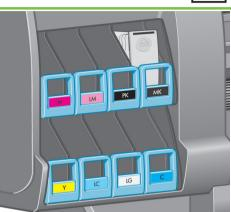
Remove the transparent shipping tray. Insert the maintenance cartridge, pushing it in
