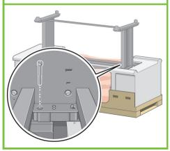
Use two screws to attach the left side of the stand to the printer. Make sure that the screws are fully tightened.
