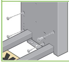
Use four screws to attach the cross-bar to the legs.
