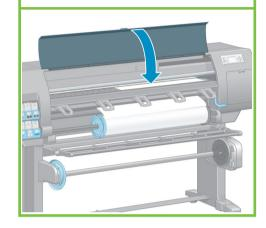
Loading roll Wind any excess paper onto roll to ensure image quality when printing. Press wk to continue
