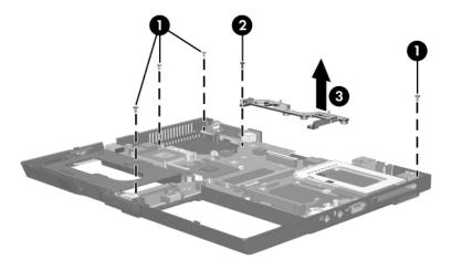
Removing the System Board Screws
