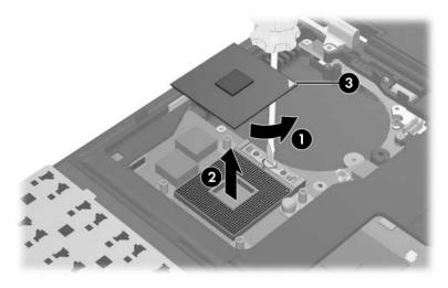
Removing the Processor
