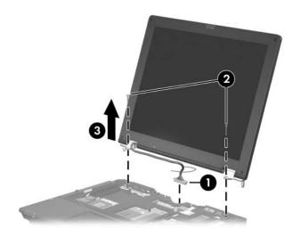
Removing the Display Assembly
