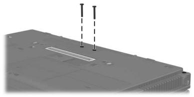
Removing the Keyboard Cover Screws
