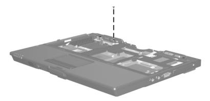
Removing the Top Cover Screw, Part 2
