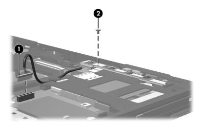
Removing the Button Board Screw
