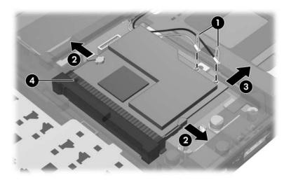
Removing a Mini PCI Communications Card
