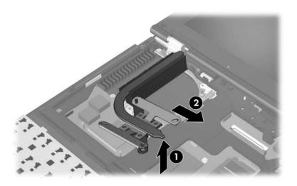
Removing the Heat Sink
