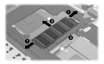
Removing the Internal Memory Module
