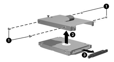
Removing the Hard Drive Frame
