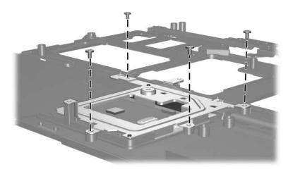
Removing the TouchPad Bracket Screws
