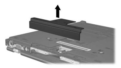
Removing the Base Enclosure Cover
