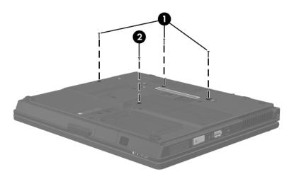
Removing the Keyboard Screws
