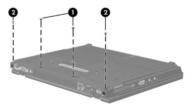
Removing the Display Assembly Screws
