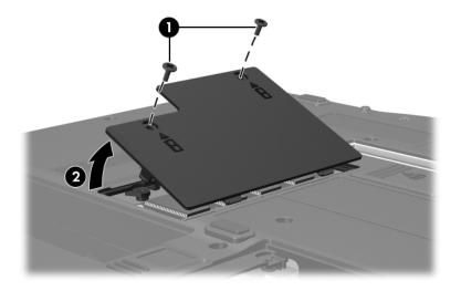
Removing the Memory Module Compartment Cover
