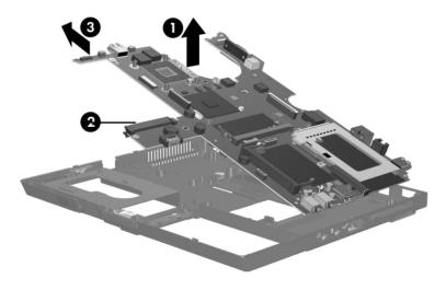
Removing the System Board
