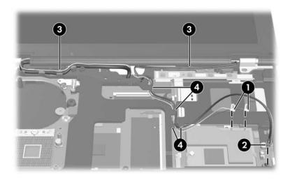
Disconnecting the Display Cables
