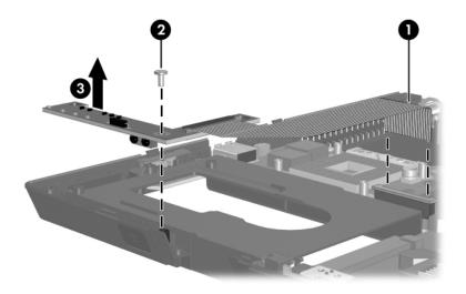
Removing the Infrared Board
