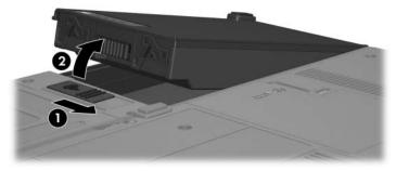
Removing the Battery Pack
