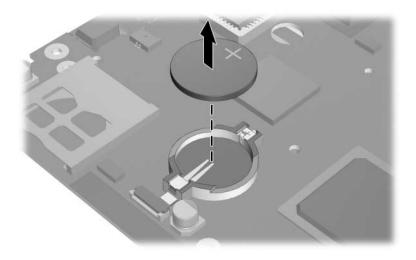
Removing the RTC Battery
