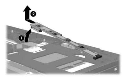
Removing the Button Board
