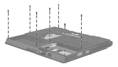
Removing the Top Cover Screws, Part 1
