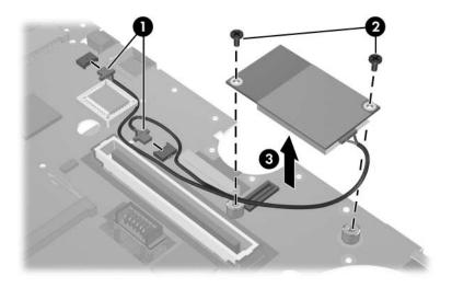
Removing the Modem Board
