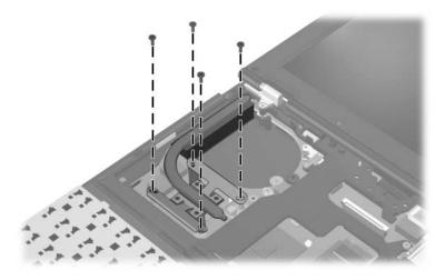
Removing the Heat Sink Screws
