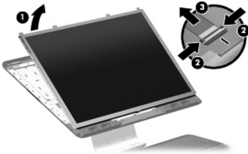
20. Remove the display panel. The display panel is available using spare part numbers 452301-001 (20.1-inch, WSXGA+BrightView) and 452302-001 (20.1-inch, WUXGA).
