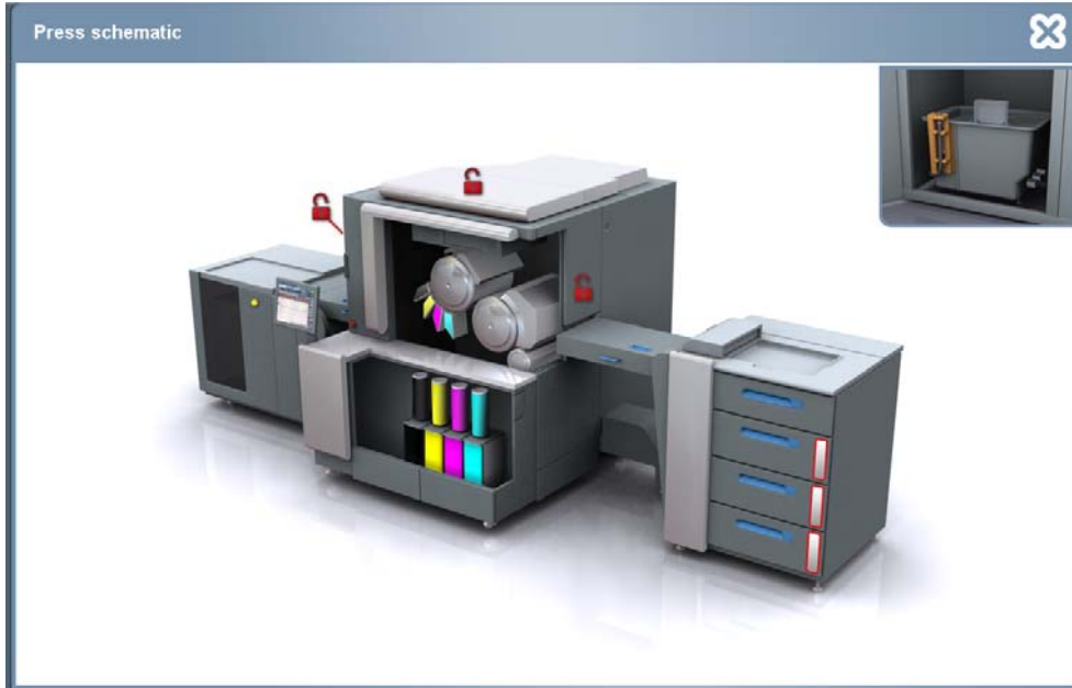
Figure 3-5 Press schematic showing open interlock doors
