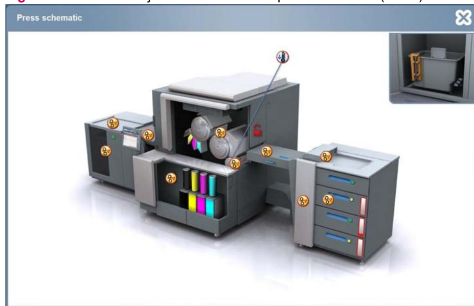
Figure 7-10 Substrate jam indicators on the press schematic (2 of 2)
