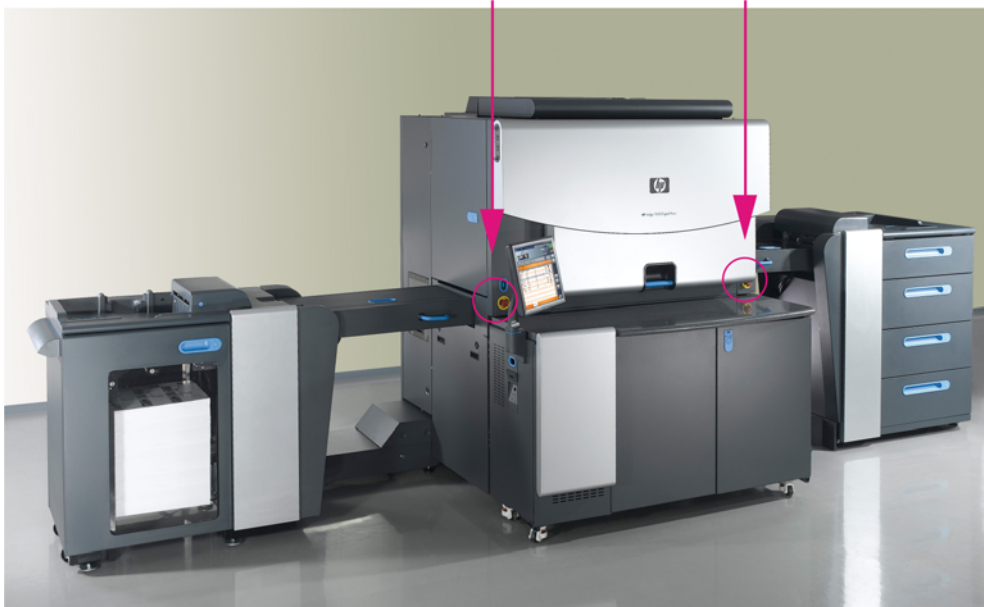
Figure 3-1 Emergency Stop button on right and left sides of front door
